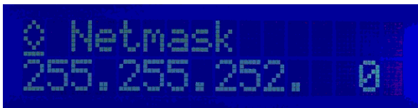
Figure 6 Subnet mask of the HCU200
