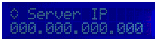
Figure 9 IP address of the PathTrak server that this HCU200 is connected to (This will change/update when the HCU200 is added to a new server)
